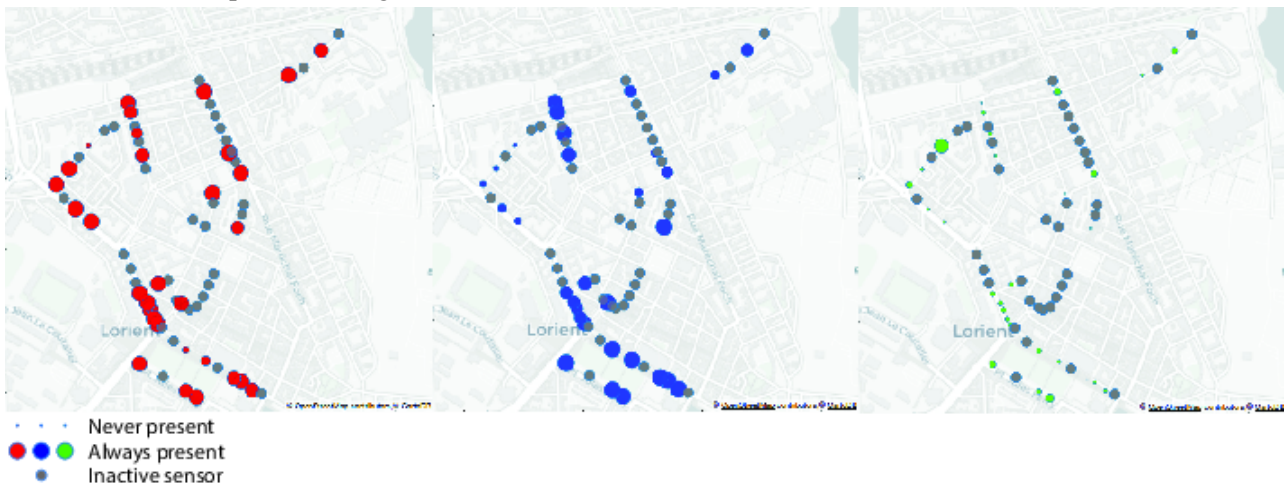
Fig. 9: Estimation of the time of presence of traffic (red), voice (blue), and birds (green) from spectral data using deep learning techniques
